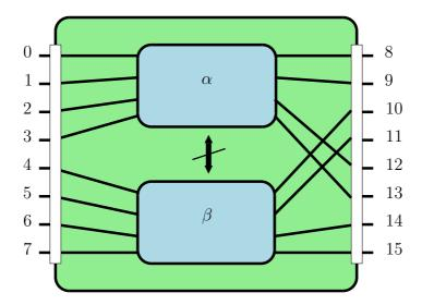
Figure 10: Example of optimal configuration for a  $8\times8$  T-switch of type va considering the forward and turnaround connections.
