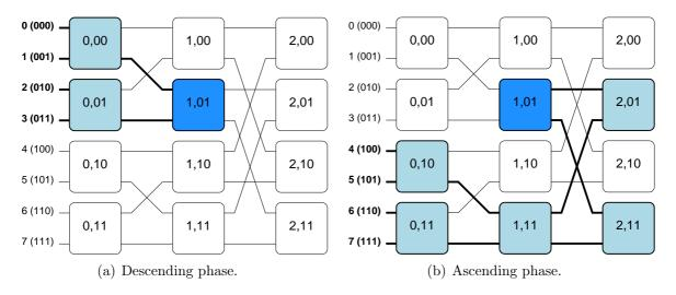
Figure 3: Reachable nodes from a switch considering the topology.
