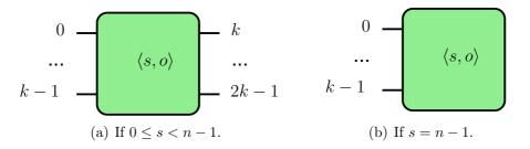
Figure 25: Numbering scheme for switch ports.
