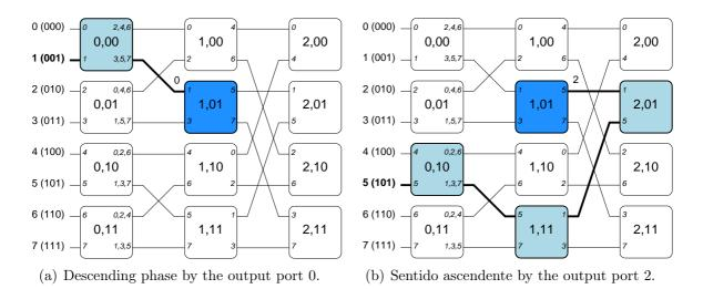
Figure 6: Reachable nodes through a port from a switch considering the routing algorithm.
