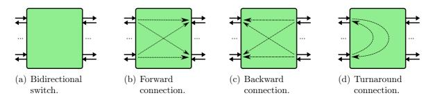
Figure 20: Internal connections in a bidirectional switch.
