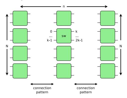
Figure 16: Assumed notation for a MIN with N terminals and  $k \times k$  switches.
