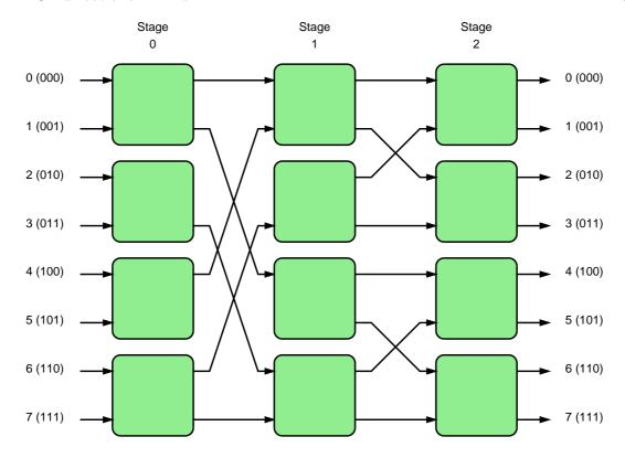
Figure 18: Unidirectional MIN built with  $2\times 2$  switches.
