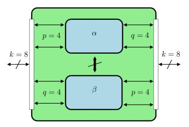
Figure 9: Optimal configuration of a  $8\times8$  T-switch of type va considering forward and turnaround connections.
