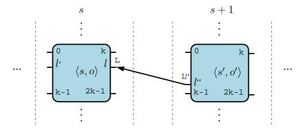
Figure 7: Associated channel between two adjacent switches.
