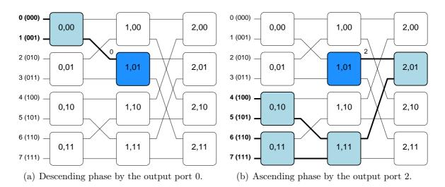
Figure 4: Reachable nodes through a port from a switch considering the topology.
