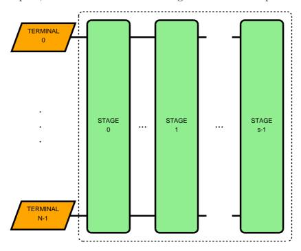
Figure 14: A multistage network with N terminals and s stages.
