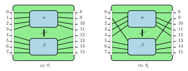
Figure 11: Optimal switch configurations for a  $8\times8$  T-switch considering backward connections.
