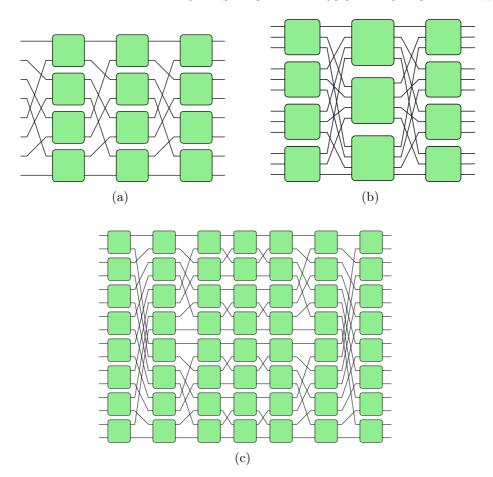
Figure 15: MINs: (a) Omega  $8\times8$ , (b) 3–stage Clos, (c) Benës  $8\times8$ .
