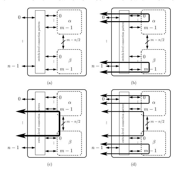
Figure 1: (a) Basic block diagram of a T-switch and several cases: (b) Optimal, (c) Bad, and (d) General.
