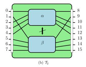
Figure 12: Possible optimal configurations for a  $8\times8$  T-switch of type va considering backward connections.
