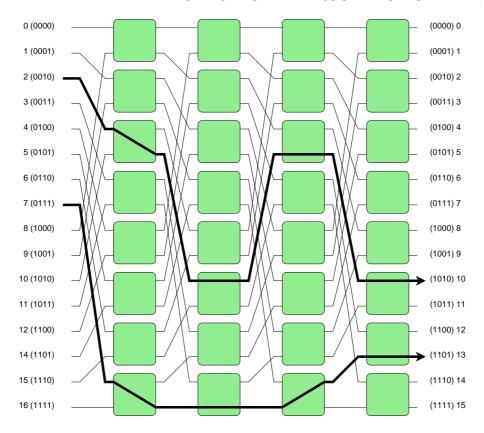
Figure 19: Paths selected by the self-routing algorithm in a N=16 butterfly MIN.
